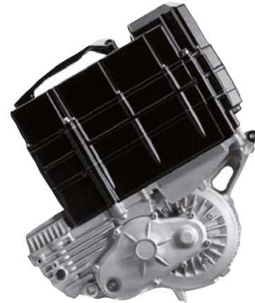
Fully integrated PMS Motor of KTM E-Enduro Freeride E-XC
